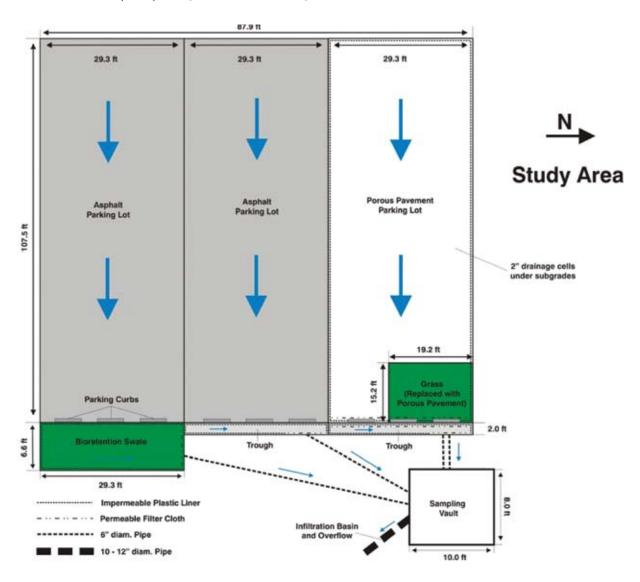
Figure 1. The Seneca College test site evaluates runoff directly from asphalt, from asphalt into a bioswale as well as surface and subsurface runoff from permeable interlocking concrete pavement.
