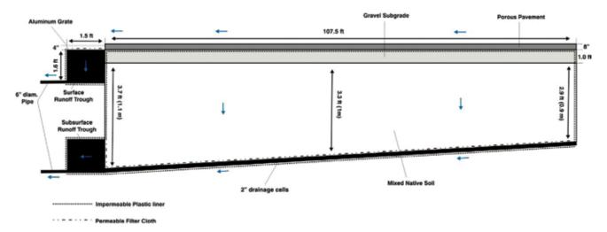
Figure 3. The PICP test area includes subsurface monitoring at the bottom of the open-graded base and further down within the soil subgrade. Water is sampled inside the troughs or utility vaults.
